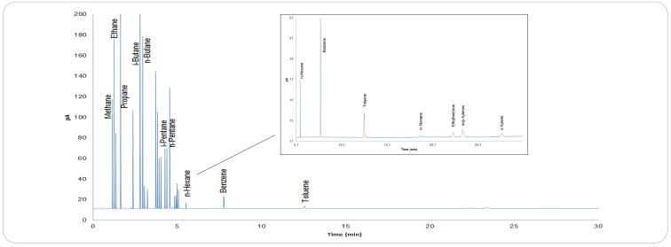
Hi-Speed RGA in Extended Mode allows Analysis of BTEX
