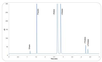
LPG Sample Analysis using the Hi-Speed RGA
