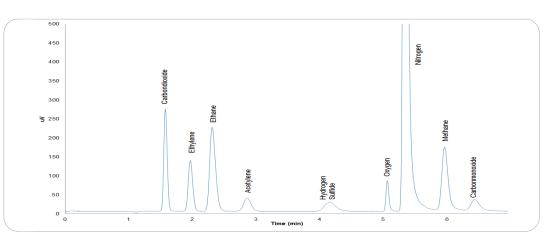
Permanent Gases and Hydrogen Sulfi de Channel
